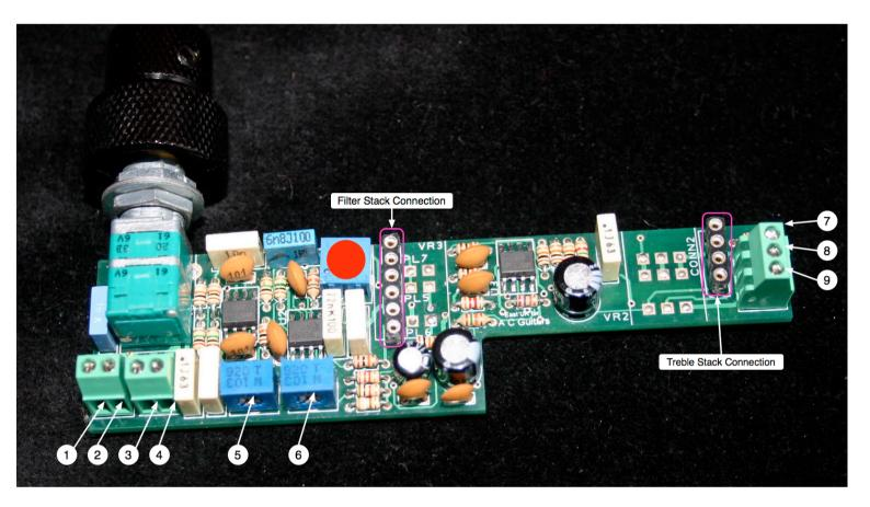
This board is common to all configurations. Filter stack connection is now duplicated on the reverse of the board.
